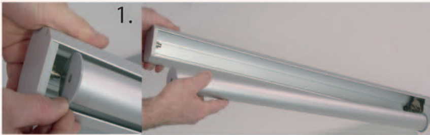
Take Motorized Revolving unit and push on the inside roller against the retaining spring so the roller can be removed.
