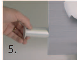
Once the roller is removed from the Motorized Revolving Unit slide it inside of the graphic loop.
